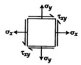
Determine the direction and magnitude of principal stresses in the material.
