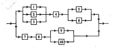
Assume that all components are independent and reliability of each component is given for a mission of 100 hours as follows:
