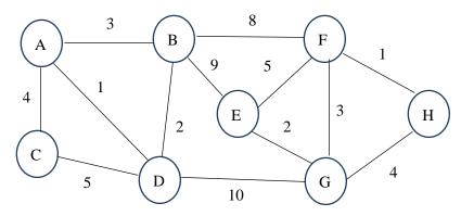
Q4. Apply Dijkastra's Algorithm to find the shortest path from source vertex 'A' to all other vertices for following graph.
