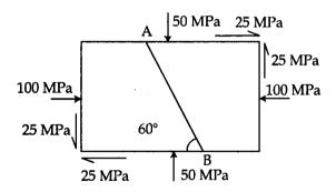
Find the normal and shearing stresses on the section AB inclined at an angle of 60° with (x-x) axis. Also find the resultant stress on the section.
