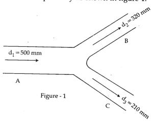
If the average velocity in 500 mm diameter pipe is 3.2 m/sec, find :
