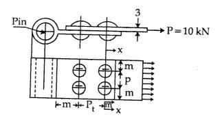
A brake band attached to the hinge by means of a riveted joint is shown in the figure. Determine the size of the rivets needed for the load of  $10 \, \text{kN}$ . Also determine the width of the band. The permissible stresses for the band and rivets in tension, shear and compression are 80, 60,  $120 \, \text{N/mm}^2$  respectively. Assume margin (m) =  $1.5 \, \text{d}$ .
