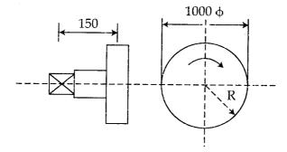
A line shaft transmits 25 kW power at 200 rpm by means of a vertical belt drive. The diameter of the belt pulley is 1000 mm and the pulley overhangs 150 mm beyond the centre line of the end bearing. The belt tensions acts vertically downwards. The tension on the tight side of the belt is 2.5 times that on the slack side. The shaft is made of plain carbon steel 40 C 8 (Syt = 380 N/mm²) and the Factor of safety is 2.5. The mass of the pulley is 25 kg. Determine the diameter of the shaft.
