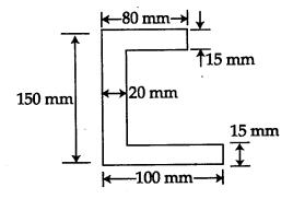
(b) Find the moment of inertia about the horizontal centroidal axis and about its base AB.
