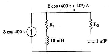
(b) Determine the input admittance, Y<sub>in</sub>, in the following circuit:
