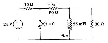
(b) In the following circuit, the switch is opened at time, t = 0. Determine  $v_c$  as a function of time.
