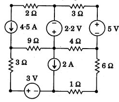
(b) Determine the current i<sub>x</sub> in the following circuit:
