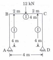
**4.** Find the moment at the supports of the continuous beam shown in the figure. The beam is of uniform section.
