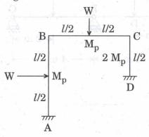
6. The axial and flexural rigidities of the members of a plane frame shown in the figure are EA and EI respectively. Joint B is free to translate and rotate. Calculate the stiffness coefficients corresponding to the three displacements shown in the figure and assemble the stiffness matrix.
