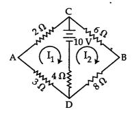
(b) Use Superposition theorem to find currents in various branches of the circuit.
