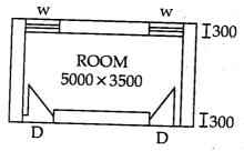
Note : All dimensions are in mm  $W = 1000 \times 1200 \text{ mm}$  $D = 1000 \times 2100 \text{ mm}$
