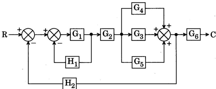
3. The block diagram of an electronic pacemaker is given below. Determine the steady state error for unit ramp input when  $k = 400$ . Also determine the value of  $k$  for which the steady state error to a unit ramp will be 0.02.
