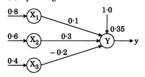
**3.** (a) Find the weights required to perform the following classification using perceptron network:
