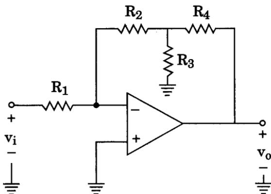
Use this circuit to design an inverting amplifier with a gain of 100 and an input resistance of 1 M $\Omega$ . Assume that for practical reasons it is required not to use resistors greater than 1 M $\Omega$ .
